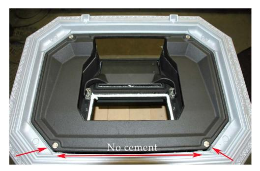
5. Firmly press the gasket into the stove cement in the channel. It may be necessary to stretch or compress the gasket, as the gap of the channel can be narrower or wider. Use a putty knife to fully seat the gasket.
