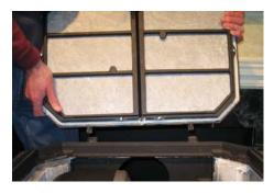
3. Use a putty knife or flat blade screwdriver to remove the old gasket and cement from around the perimeter of the air duct cover. Remove any residual gasket and cement with a wire brush and vacuum. Do not allow any debris to fall through the gap at the front of the stove, as it may obstruct the air-wash.
